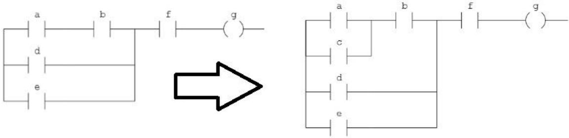
Figure 12 Contact "c" has been added
