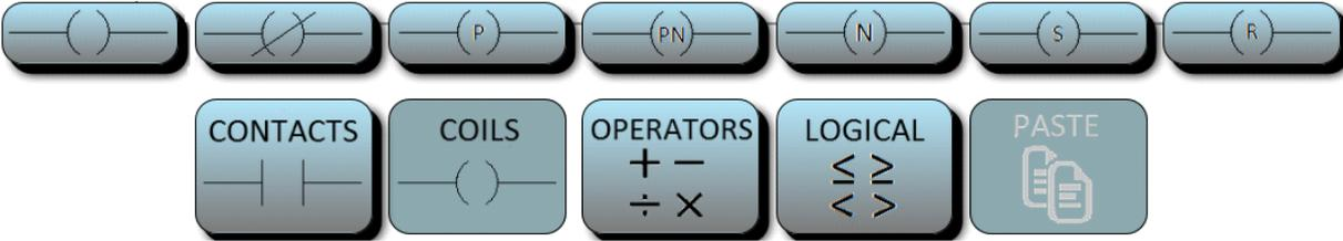
Figure 26 Showing the different elements in the sub-category "Coils"
