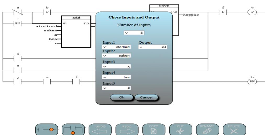
Figure 18 A menu is displayed where the user can select the inputs and outputs
