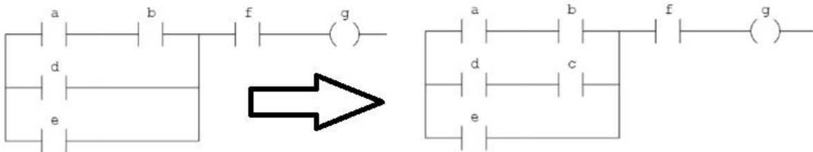
Figure 11 Contact "c" has been added
